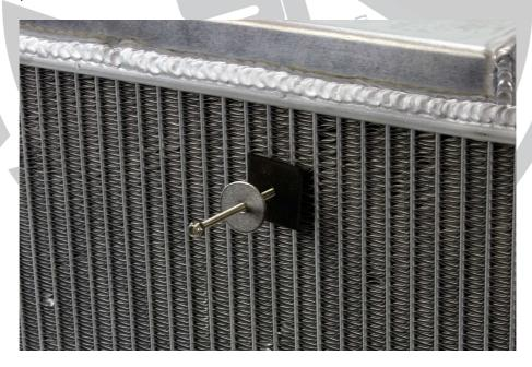
5) Repeat the process for the other three mounting brackets and then tighten each wing nut so the fan is held securely with no movement. Avoid over-tightening as this can damage the radiator core, particularly with soft metals like aluminium. Any excess mounting bolt can be cut with a dremel-type tool or hacksaw, but take care not to ruin the thread in case you need to remove and refit the fan at any point.
