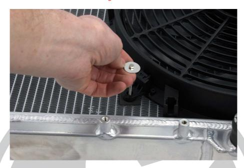
4) On the opposite side push a foam pad onto the mounting bolt, followed by a washer, and then screw on the nylon-locking nut, tightening lightly so it loosely holds the fan until the other mounting roads are in place.
